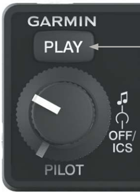
Left Knob - Pilot Volume Controls
