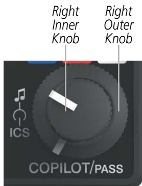
Right Knob - Copilot and Passenger Volume Controls
