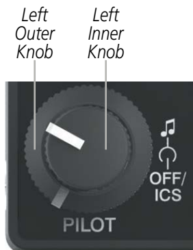
Left Knob - Pilot Volume Controls
